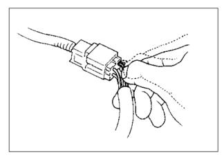
• When taking measurements at electrical connectors using a tester probe, be sure to insert the probe from the wire harness side (backside) of the connector / coupler.
