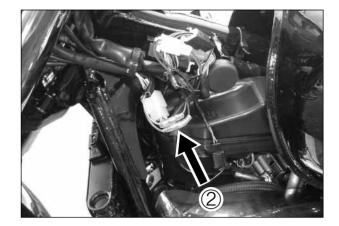
7) Measure the voltage between (18) of the ECU and the LY wire of the wiring harness's GP switch coupler, and measure the voltage between (18) of the ECU and the GR wire of the wiring harness's clutch lever switch coupler.
