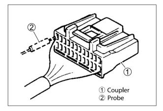
When connecting meter probe from the terminal side of the coupler (connection from harness side not being possible), use extra care not to force and cause the male terminal to bend or the female terminal to open.
