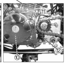
10 Magneto11 Pick-up coil12 GP switch
