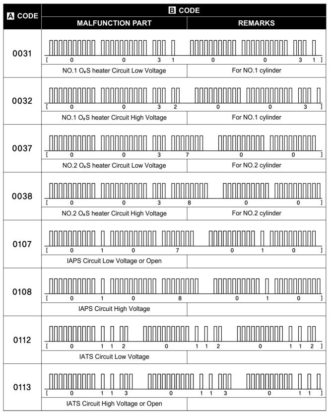
\* A CODE : For LCD (DISPLAY) indication [Applies only to GT250/P/ REIDSON]]
