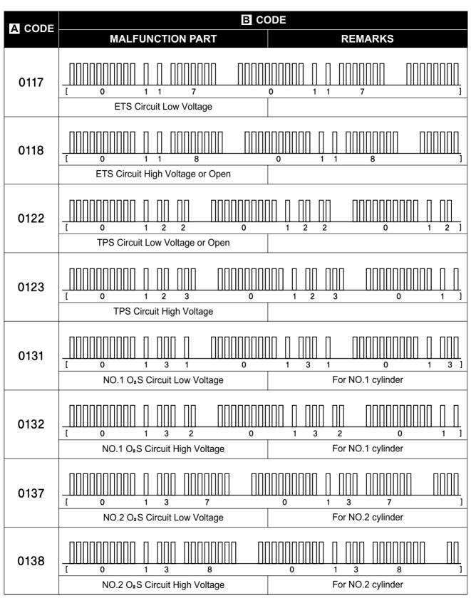
\* A CODE : For LCD (DISPLAY) indication [Applies only to GT250/P/REIDSOC]]
