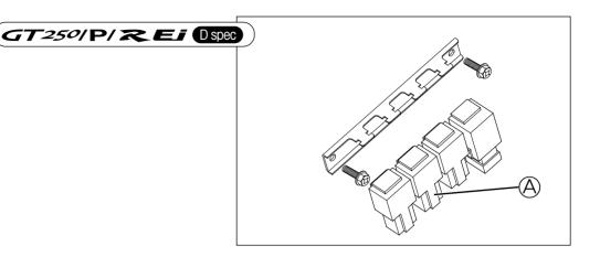
First, check the insulation between ① and ② terminals with the pocket tester. Then apply 12 volts to ③ and ④ terminals, ⊕ to ③ and ⊖ to ④, and check the continuity between ① and ②.
