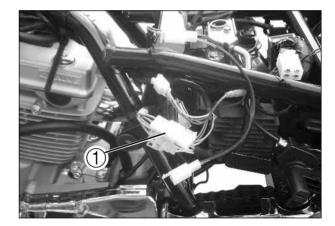
4) Disconnect the pick-up coil coupler ① and measure the resistance.
