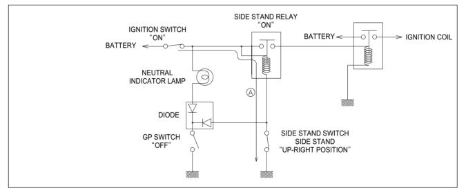
" GV250 EI DSPCC & " GT250/P/ REI DSPCC , are equipped with the side stand ignition interlock system.
